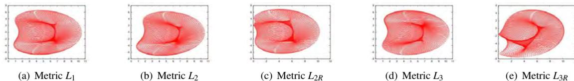
Figure 6: Cross-sectional area of the workspace of the robot manipulator considering the Global Criterion Method
