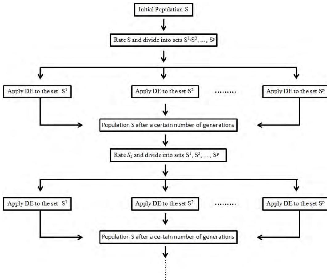
Figure 1: Flowchart of Improved Differential Evolution Method
