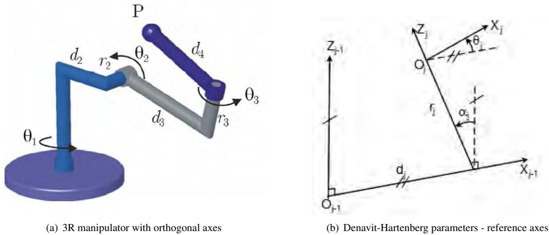
Figure 3: Representation of Denavit-Hartenberg parameters to 3R manipulator
