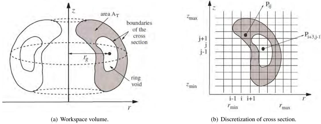
Figure 4: A scheme for evaluating the workspace volume of 3R manipulators and discretization of the cross section area by using a rectangular mesh.
