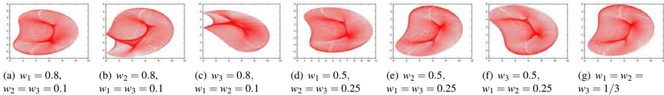
Figure 5: Cross-sectional area of the workspace of the robot manipulator considering the Weighting Objectives Method
