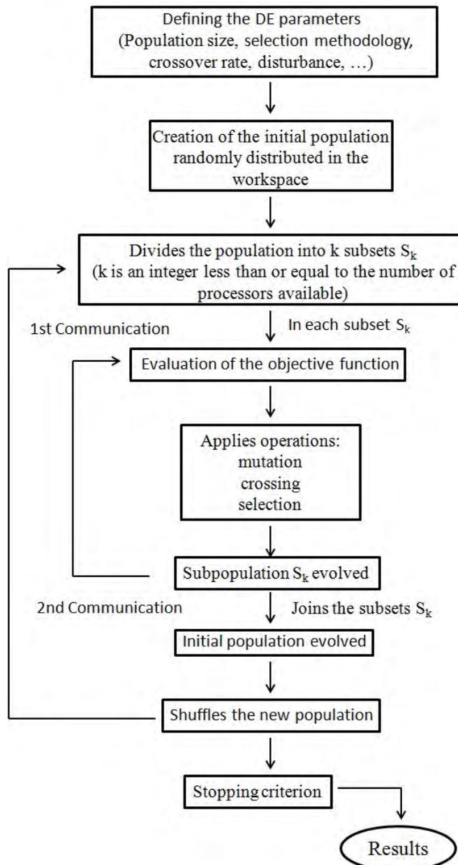
Figure 2: Flowchart of Improved Differential Evolution Algorithm with Parallel Processing
