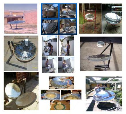
Figure 1. Solar cookers manufactured and tested in LMHES / UFRN.
