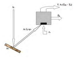
Figure 4. Energy flow-capture system converting solar radiation into heat energy.
