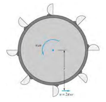
Figure 3. Schematic Design of the Water Wheel used for White F. M. (1999).
