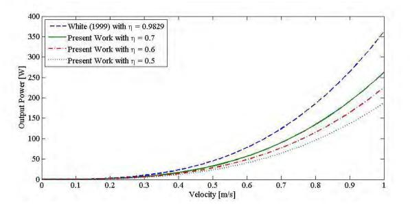
Figure 11. Power output as a function of Velocity, using the various values of performances.
