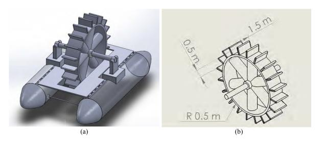
Figure 2. (a) Schematic drawing of floating the water wheel. (b) Schematic drawing of the water wheel dimensions.
