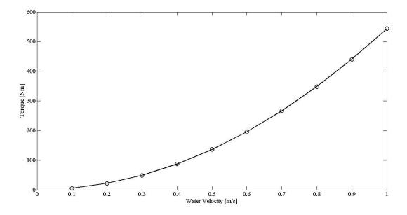
Figure 7. Torque as a function of water velocity
