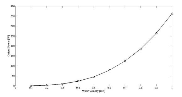
Figure 6. Output power as a function of velocity.
