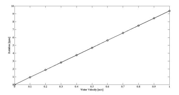
Figure 8. Rotation as a function of water velocity
