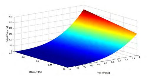
Figure 9. Power output as a function of Velocity and Efficiency, using the proposed model.
