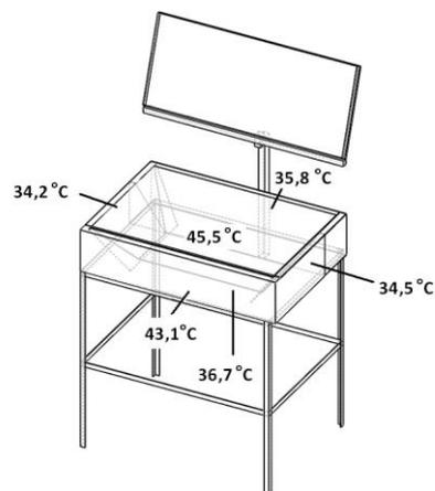
Figure 7. Temperatures on the external surfaces of the oven.
