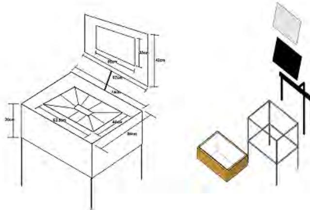
Figure 2. Schematic drawing of the solar oven, its components and its dimensions.
