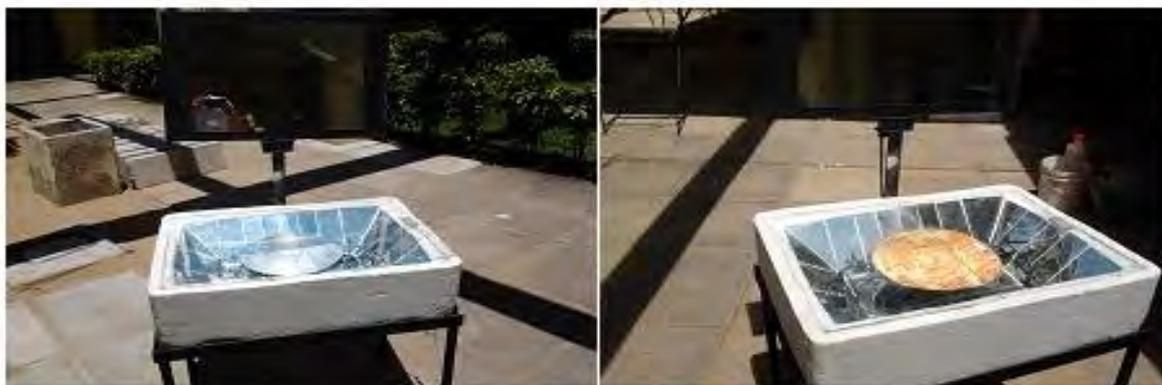
Figure 3. Solar oven proposed in test in Solar Energy Laboratory UFRN.
