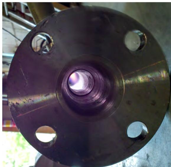
Figure 6. Electric arc working inside the Venturi
