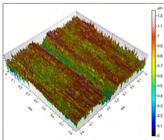
Figure 1. General topography on the work surface.
