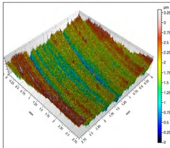
Figure 2. General topography on the electrodes' surfaces used in the experiments.
