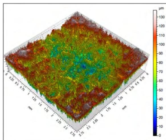
Figure 3. General topography on the EDM machine surfaces.
