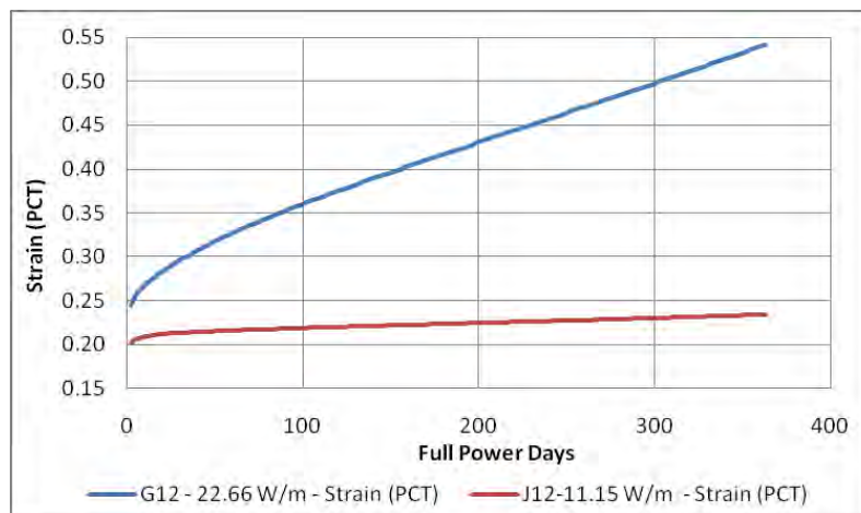
Figure 13: Temporal evolution of the cladding axial strain thickness of the fuel rods simulated with FRAPCON code
