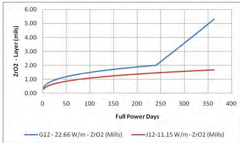
Figure 11: Temporal evolution of the ZrO_2 thickness in the cladding of fuel rods simulated with the FRAPCON code
