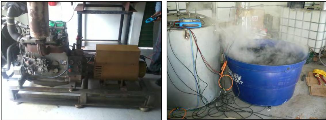
Figure 3. Diesel engine MWM D229-4, generator KOHALBACH and liquid resistance - Charge simulation
