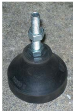
Figure 1. Adjustable support used as table foot.
