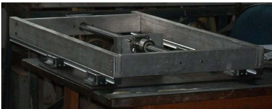
Figure 7. Bottom view of the bench with the spindle and the chestnut of the base of the table.
