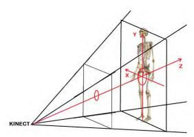
Figure 4. The coordinate system of the Kinect.
