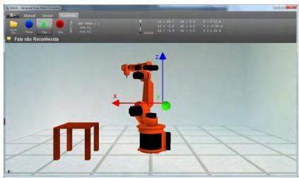
Figure 8. Robot motion based on a KRL code file.
