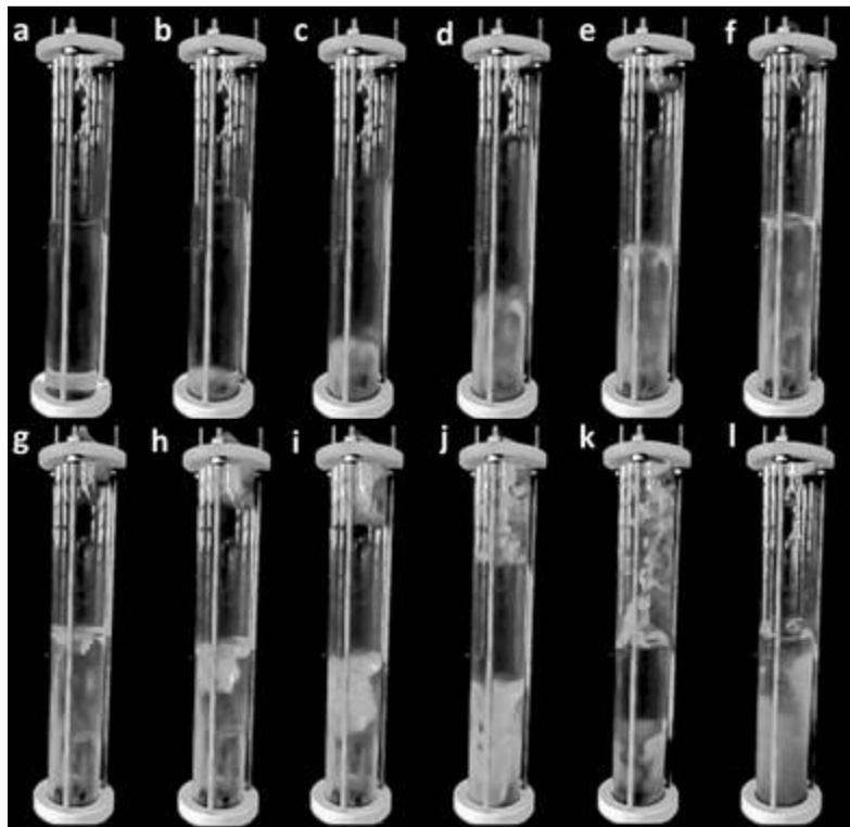
Figure 4. Expansion of the cavity and formation of the piston like movement of the water in the container.
