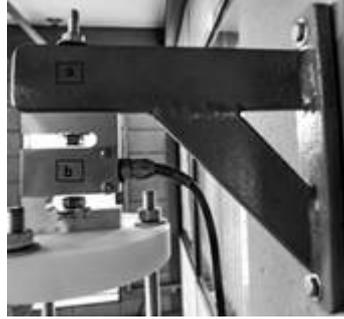
Figure 2. Bracket (a) and charge cell (b).
