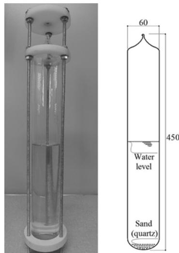
Figure 1. Water container. Dimensions in millimeters.
