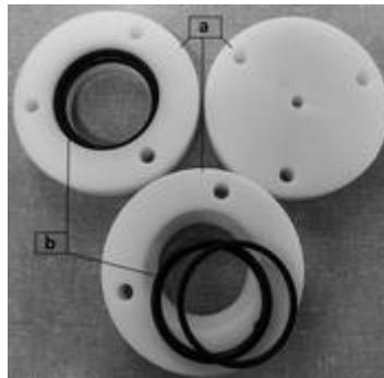
Figure 3. PVC plate and washers (a) and O-rings (b).
