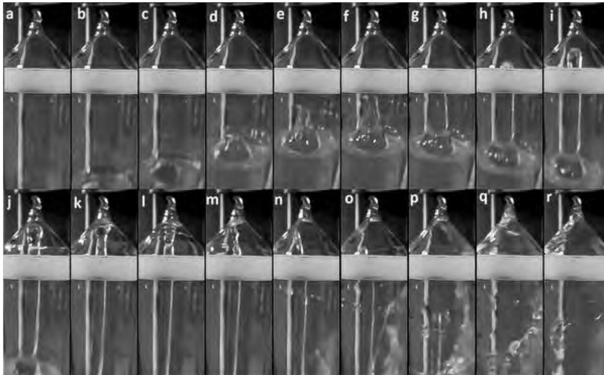
Figure 6. Formation and development of the central jet. The total time of the experiment was 343,7 ms
