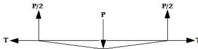
Figure 1. Representation of the forces  $T$  and  $P$  and the deflection in equilibrium condition. (Cajuhi and Batista, 2010).
