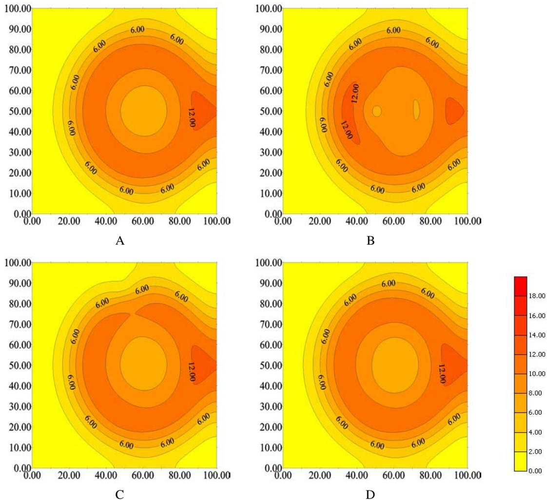
Figure 6. Amplitudes of the stress wave, varying from zero (in yellow) to nineteen (in red), with tension source in the point  $(60, 50)$  mm at time  $35$  ms in four models: (A) the homogeneous welded plate with  $c = 0.965$  m/s ; (B) the welded plate with a crack with speed  $c = 0.4$  m/s; (C) the welded plate with pores with speed  $c = 0.4$  m/s; (D) the welded plate with slag inclusion in the center of the plate with speed  $c = 1.2$  m/s.
