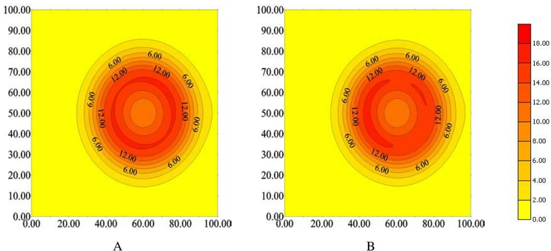
Figure 4. Amplitudes of the stress wave, varying from zero (in yellow) to nineteen (in red), with tension source in the point  $(60, 50)$  at time  $25 \text{ ms}$ , in two models: (A) homogeneous plate with speed  $c = 1 \text{ m/s}$ ; (B) the homogeneous plate with wave propagation speed  $c = 1 \text{ m/s}$  containing a weld of  $12 \text{ mm}$  with speed  $c = 0.965 \text{ m/s}$ .
