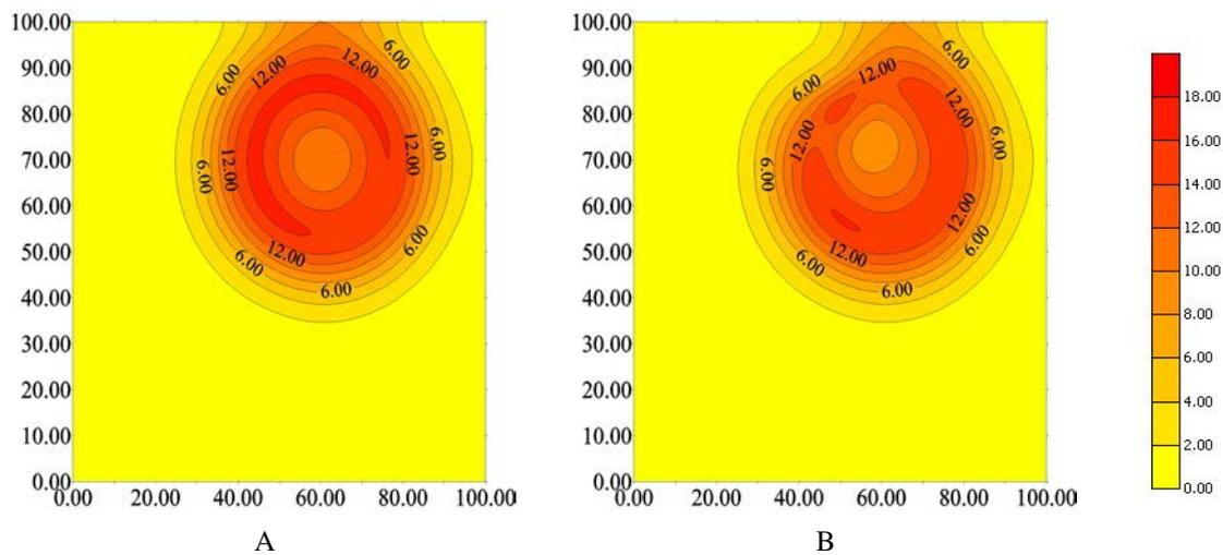
Figure 7. Amplitudes of the stress wave, varying from zero (in yellow) to nineteen (in red), with tension source in the point (60, 70) at time 25 ms in two models: (A) the homogeneous welded plate with  $c=0.965 \text{ m/s}$ ; (B) the welded plate with pores with speed  $c = 0.4 \text{ m/s}$ .
