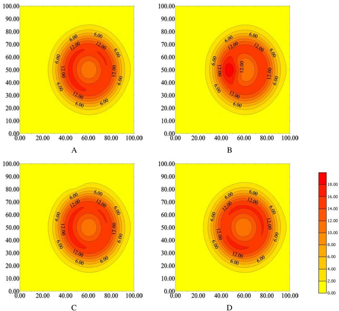
Figure 5. Amplitudes of the stress wave, varying from zero (in yellow) to nineteen (in red), with tension source in the point  $(60, 50)$  mm at time  $25$  ms in four models: (A) the homogeneous welded plate with  $c = 0.965$  m/s ; (B) the welded plate with a crack with speed  $c = 0.4$  m/s; (C) the welded plate with pores with speed  $c = 0.4$  m/s; (D) the welded plate with slag inclusion in the center of the plate with speed  $c = 1.2$  m/s.
