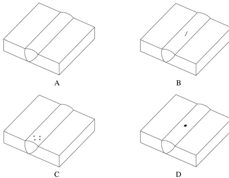
Figure 3. Homogeneous plate with wave propagation speed  $c = 1 \text{ m/s}$  containing a weld of  $12 \text{ mm}$  with speed  $c = 0.965 \text{ m/s}$ : (A) homogeneous weld; (B) plus a crack of  $4 \text{ mm}$  in the central region of the weld with speed  $c = 0.4 \text{ m/s}$ ; (C) including pores at the upper end of the weld with speed  $c = 0.4 \text{ m/s}$ ; (D) with slag inclusion in the center of the plate with speed  $c = 1.2 \text{ m/s}$ .
