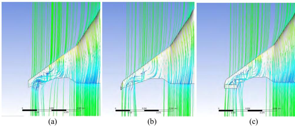
Figure 7: Visualization of small deviations for  $\alpha=8^\circ$ , (a) BWB, (b) BWB with Winglets and (c) BWB with C-Wing
