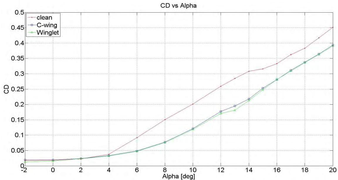
Figure 9: Variation of drag coefficient ( $C_d$ ) versus angle of attack ( $\alpha$ )
