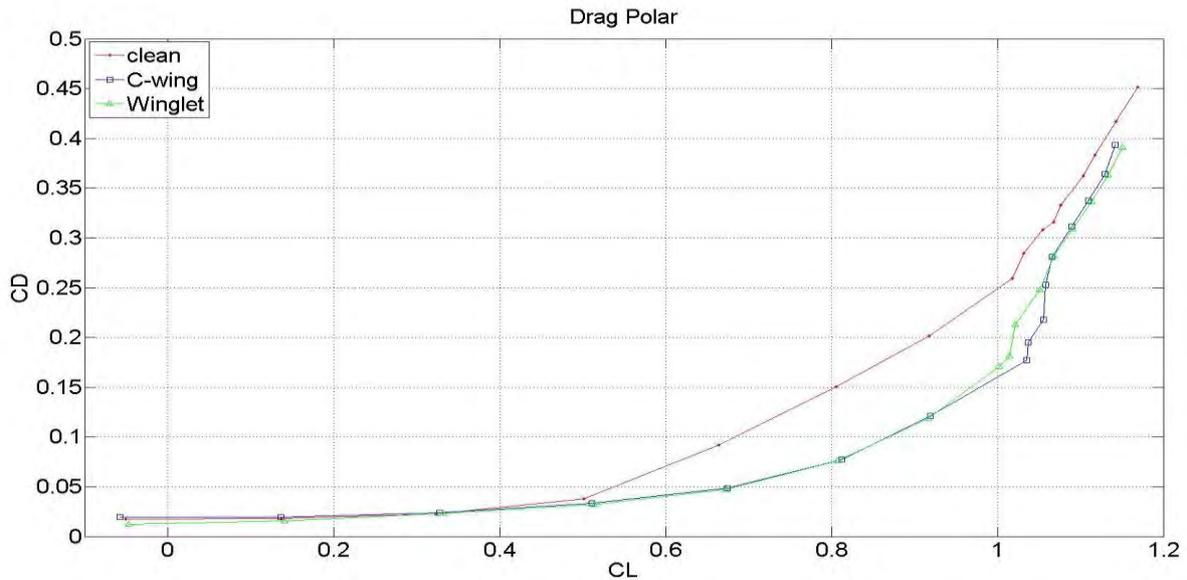
Figure 10: Drag Polar (Lift Coefficient versus Drag Coefficient) curves for three models
