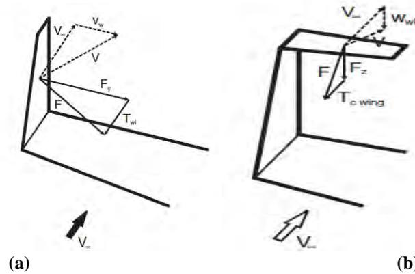
Figure 2: Schematic graph of the forces produced by the Winglets (a) and the C-Wing (b) (Slingerland and Verstraeten,2008).
