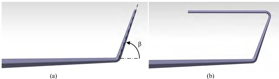
Figure 3: Wing tip devices, Winglet (a) and C-wing (b)
