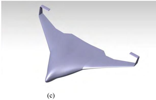
Figure 4: (a) BWB, (b) BWB with Winglets and (c) BWB with C-Wing
