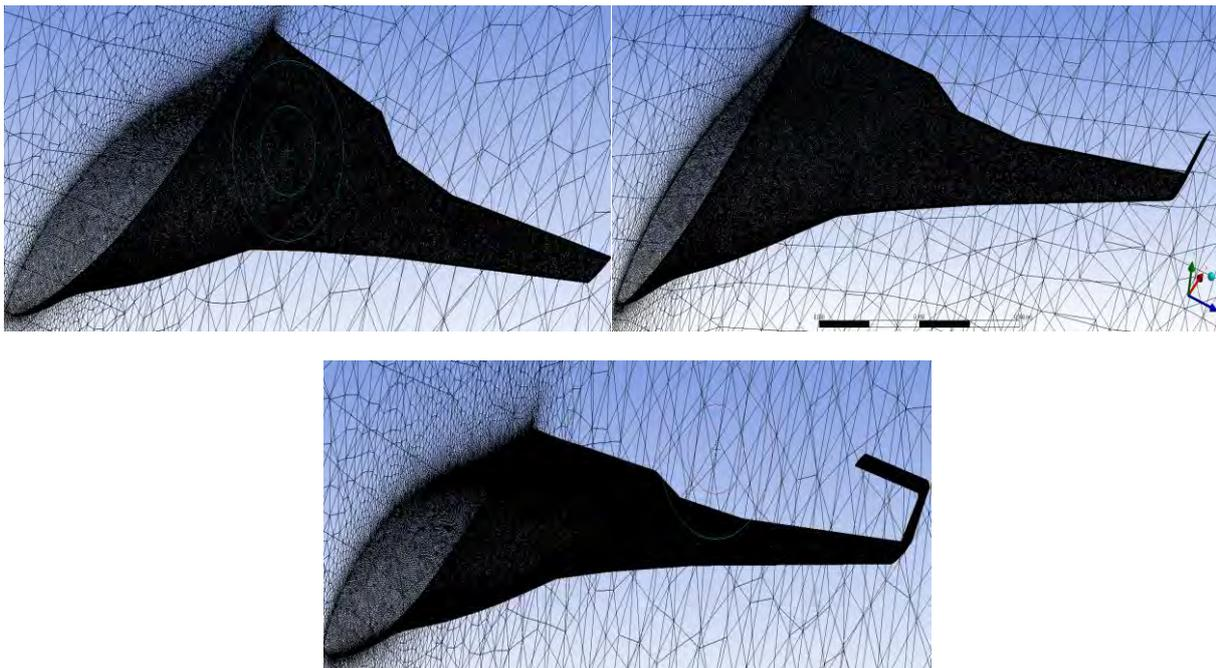
Figure 5: The wall mesh of BWB and wingtip device
