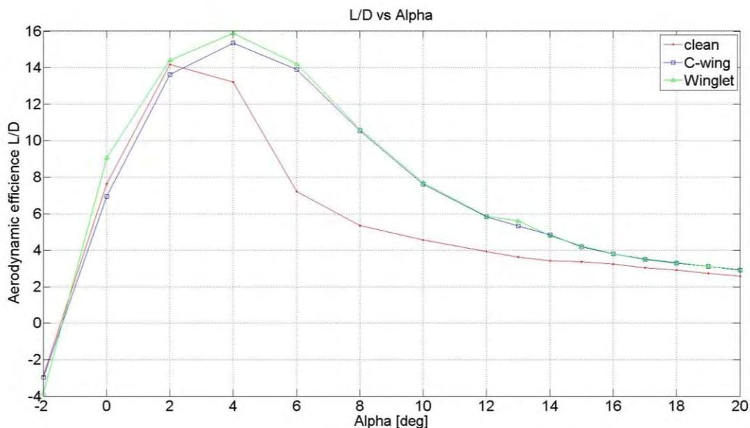
Figure 11: L/D vs Alpha curves for three models
