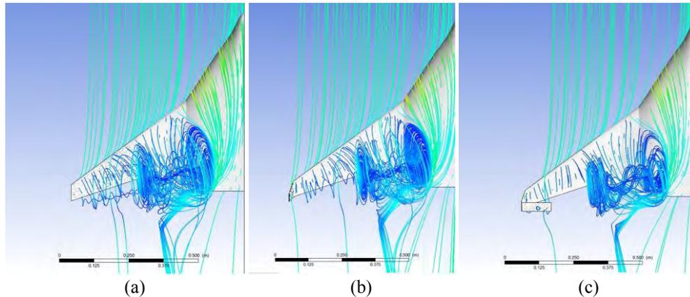
Figure 8: Visualization of small deviations for  $\alpha=20^\circ$ , (a) BWB, (b) BWB with Winglets and (c) BWB with C-Wing
