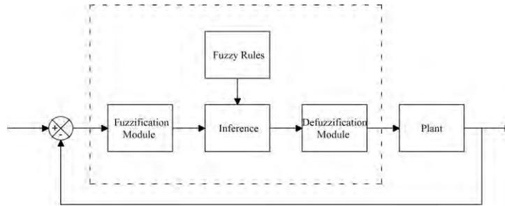
Figure 4. – Fuzzy controller block diagram
