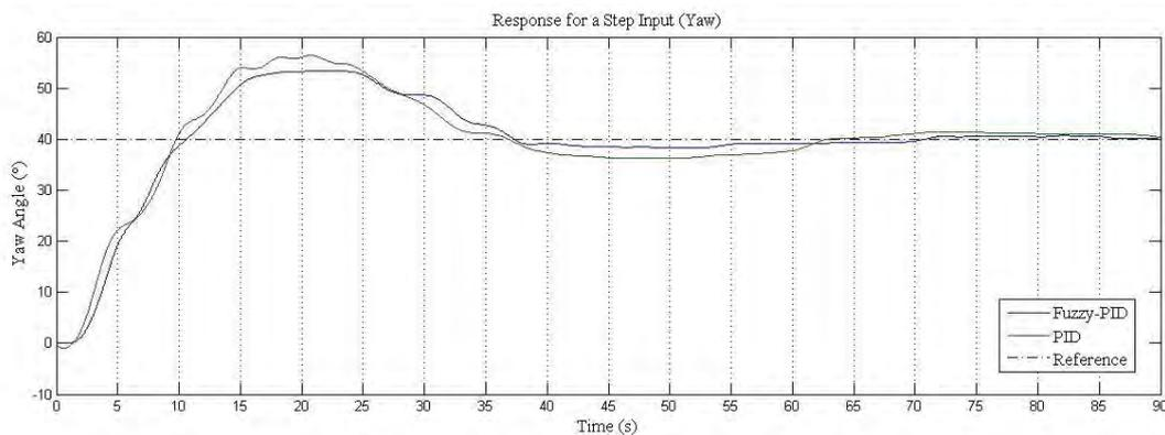
Figure 12. Diagram of the yaw response for a step input
