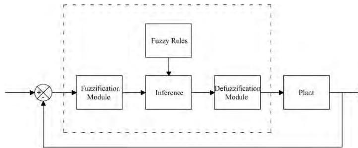
Figure 4. – Fuzzy controller block diagram
