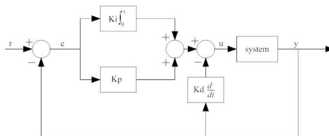
Figure 3. PI+D controller block diagram
