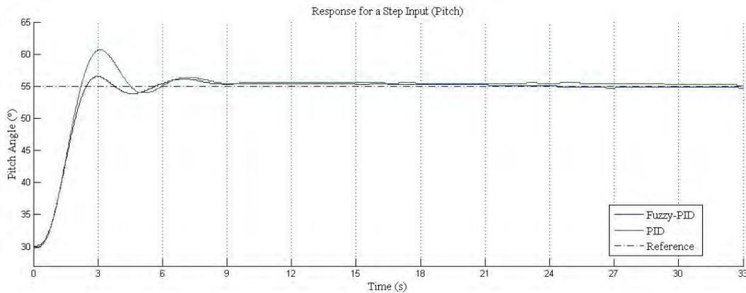
Figure 11. Diagram of the pitch response for a step input.
