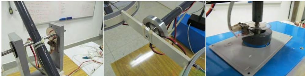
Figure 2. Encoders used for rotation angles' measurement
