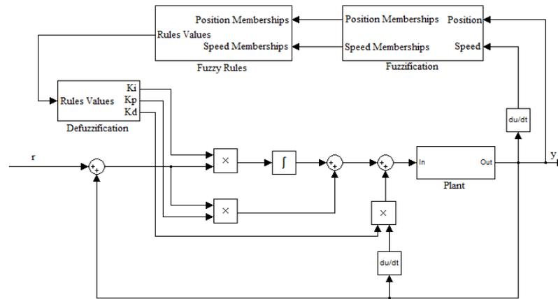
Figure 7. Fuzzy-PID controller diagram
