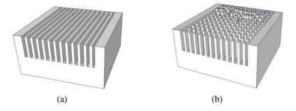
Figure 1. Enhancement structures for microchannel heat sink: (a) parallel-plate fins; (b) micro pin fins array
