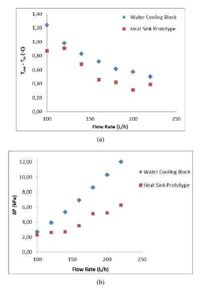
Figure 6. Comparison between results obtained by the optimized heat sink prototype and the commercial heat sink: (a) inlet and outlet temperature difference values; (b) pressure drop values
