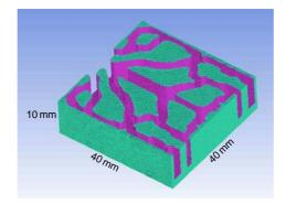
Figure 3. Geometrical model of the optimized heat sink
