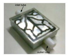
Figure 4. Manufactured heat sink prototype
