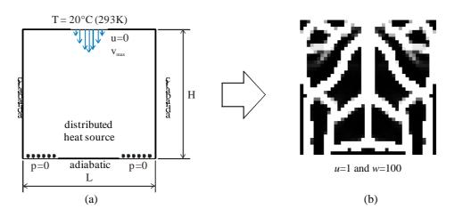
Figure 2. Topology optimization result for the heat sink design (Koga *et al.*, 2013): (a) design domain with boundary conditions; (b) result obtained for inlet velocity v<sub>max</sub> = 0.25 m/s
