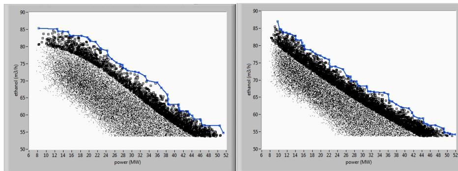
Figure 5. Operating state diagrams for two hemicelluloses conversion pathway: (a) hemicelluloses are burned, (b) hemicelluloses are fermented. Legend:  $\square$  = Pareto frontier,  $\blacksquare$  = target operating region and  $(\cdot)$  = general operating states
