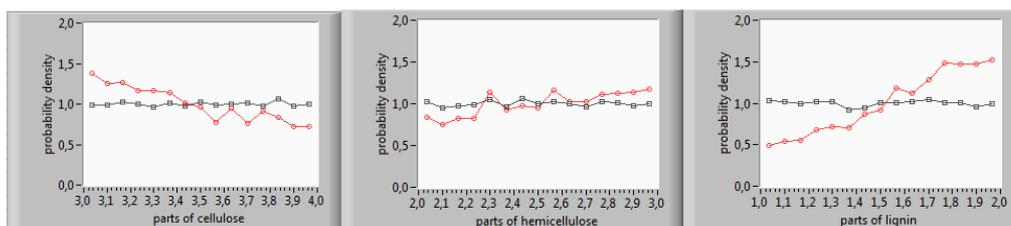
Figure 9. Fiber components probability density functions within the operating envelope ( $\square$ ) and in the optimum target region ( $\circ$ ) – hemicelluloses are burned.
