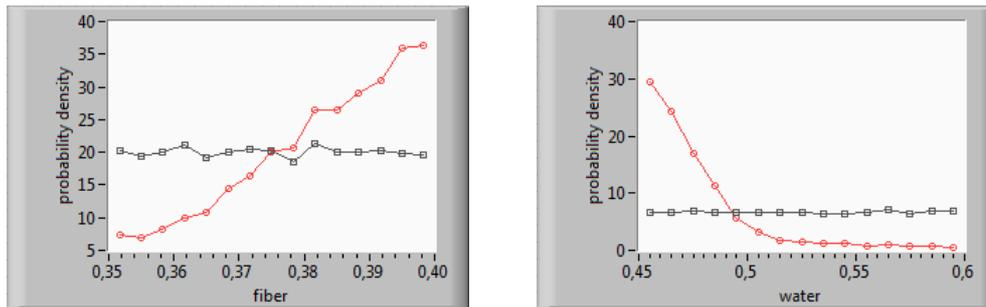
Figure 7. Fiber and water contents probability density functions within the operating envelope ( $\square$ ) and in the optimum target region ( $\circ$ ) – hemicelluloses are burned.
