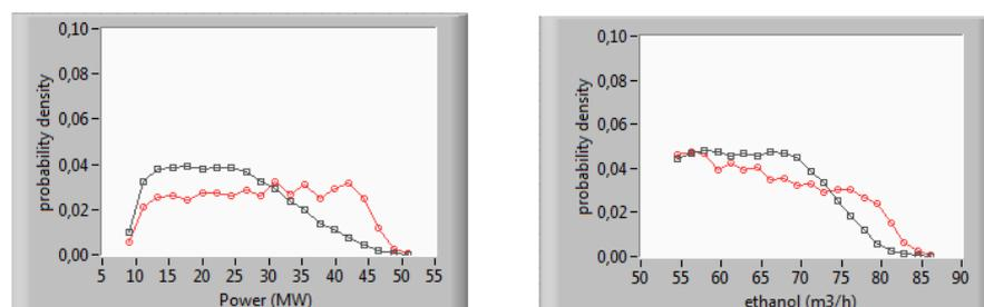
Figure 6. Power and ethanol probability density functions within the operating envelope ( $\square$ ) and in the optimum target region ( $\circ$ ) – hemicelluloses are fermented.
