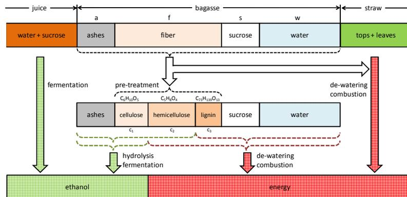
Figure 2. Sugarcane constituents conversion pathways (hemicelluloses are burned or fermented)
