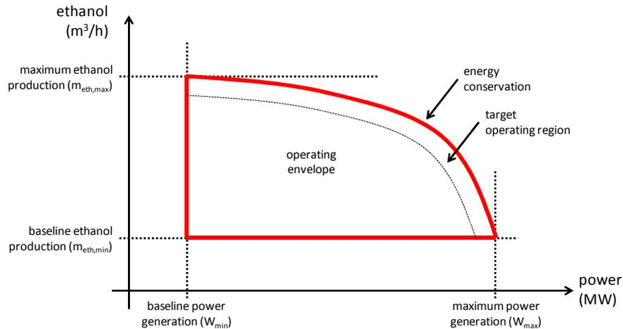
Figure 4. Ethanol-electricity graph (state diagram) and process operating envelope
