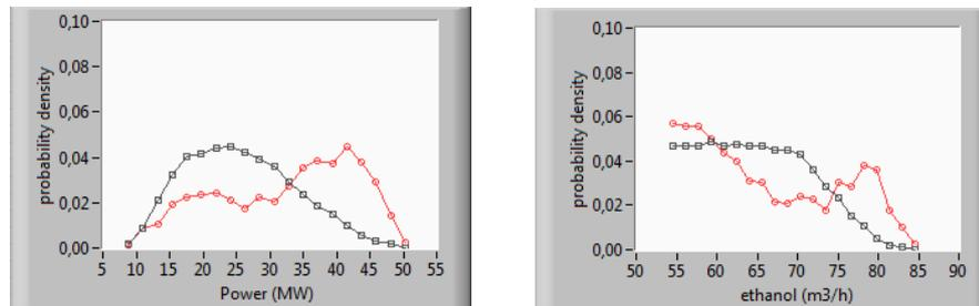
Figure 5. Power and ethanol probability density functions within the operating envelope ( $\square$ ) and in the optimum target region ( $\circ$ ) – hemicelluloses are burned
