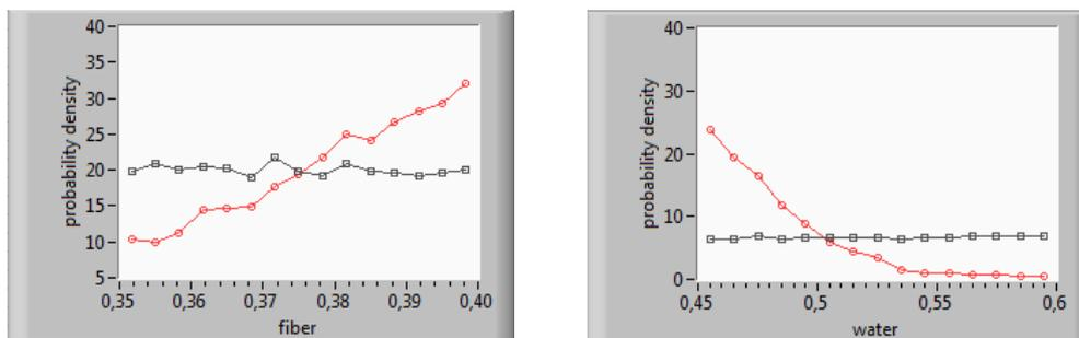
Figure 8. Fiber and water contents probability density functions within the operating envelope ( $\square$ ) and in the optimum target region ( $\circ$ ) – hemicelluloses are fermented.
