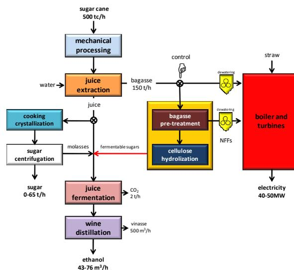
Figure 1. Reference sugarcane industrial processing model
