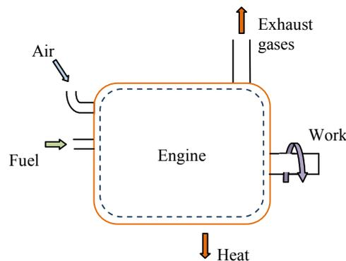
Figure 3. Control volume for the thermodynamic analysis of the diesel engine.
