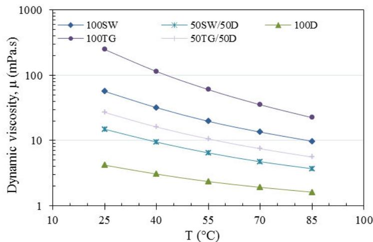
Figure 1. Dynamic viscosity of the fuels tested.
