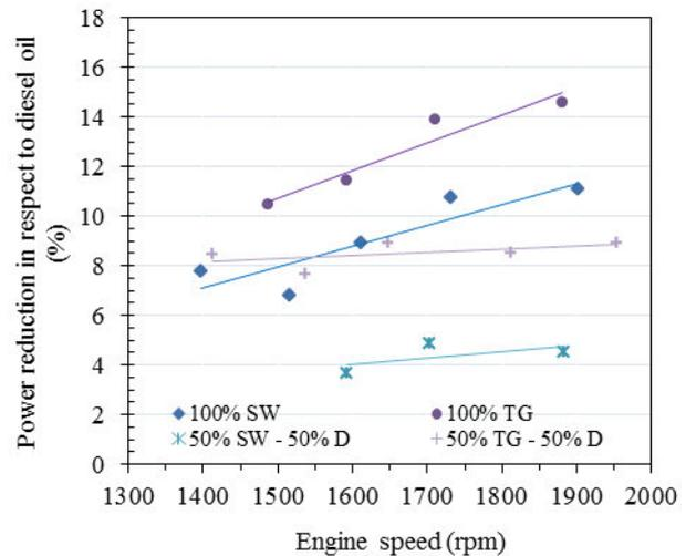
Figure 5. Power reduction in respect to diesel oil.
