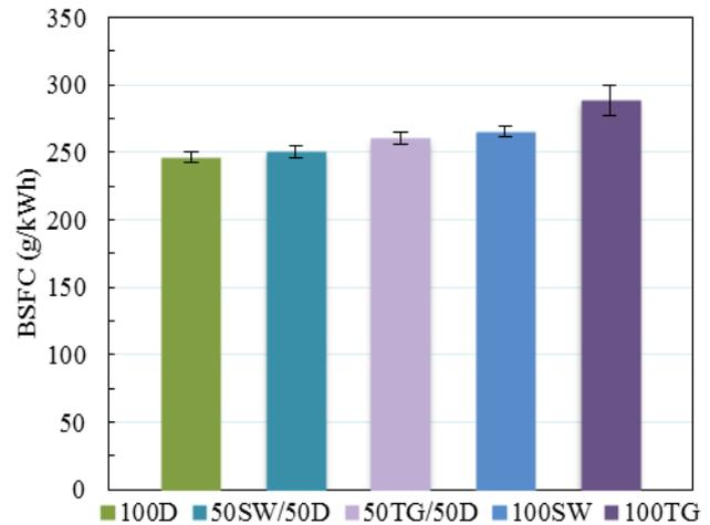
Figure 8. Break specific fuel consumption at 1800 rpm.
