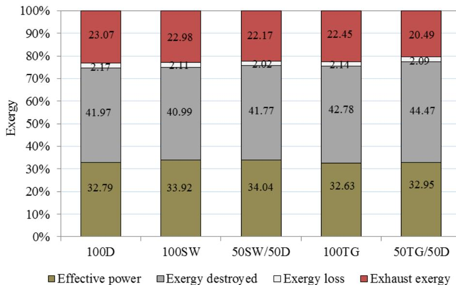
Figure 15. Exergy balance at 1800 rpm of the fuels tested.
