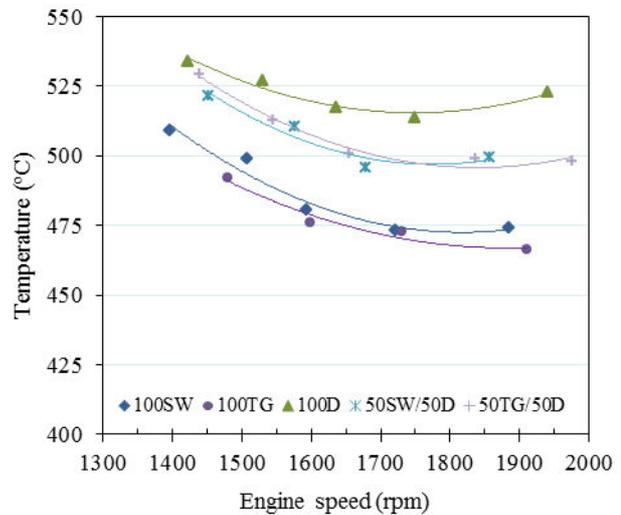
Figure 12. Exhaust gas temperature.
