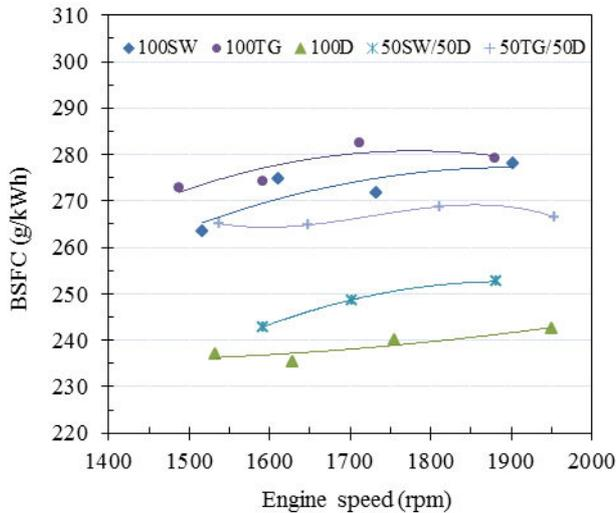
Figure 7. Break specific fuel consumption versus engine speed.
