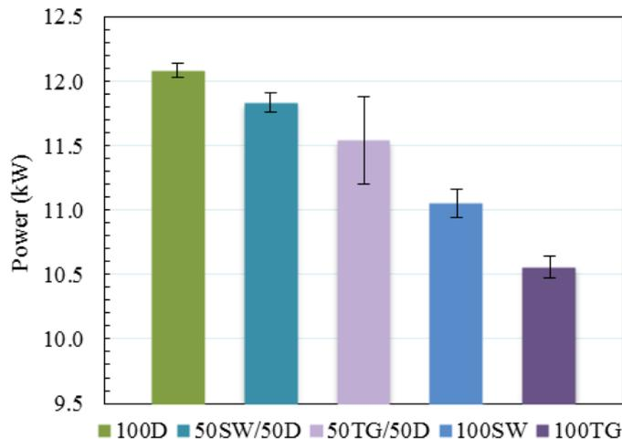
Figure 6. Power at 1800 rpm.
