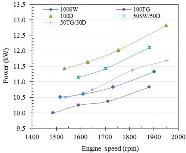
Figure 4. Power versus engine speed.
