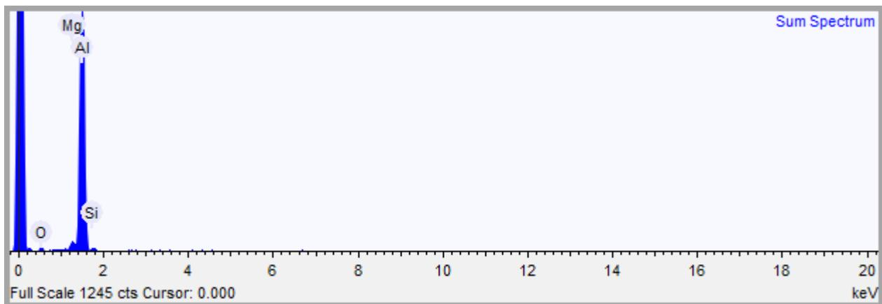
**Figure 10** - Spectrometer inclusions of the Alloy Al-2, 5wt% Mg
