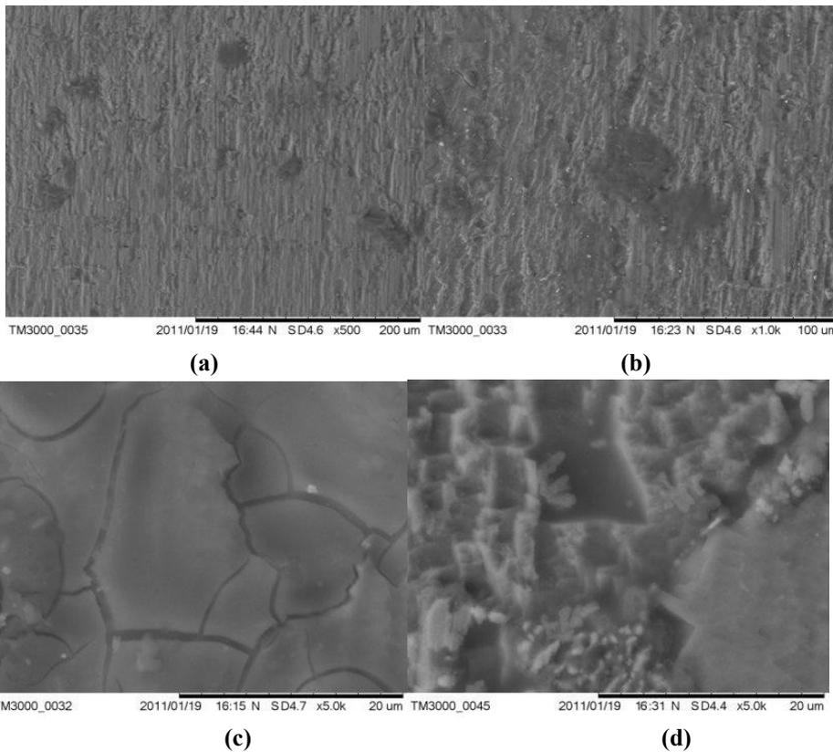
**Figure 8** - Microstructure solidified with pressure of 80 MPa (a) 500X(b) 1000X (c) 5000X (d) 5000x. MEV
