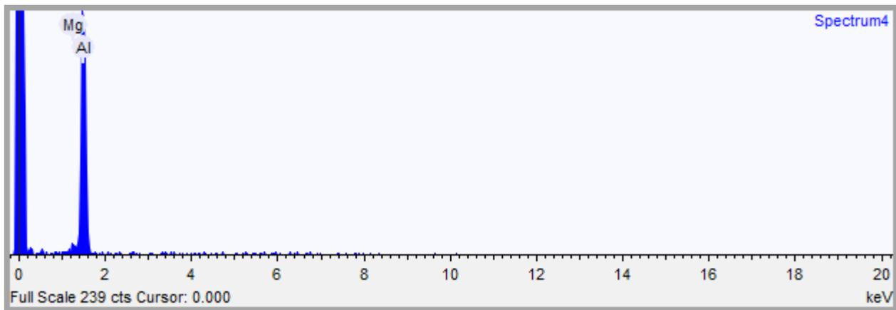
Figure 3 – Spectrometer of the Alloy Al-2, 5wt% Mg
