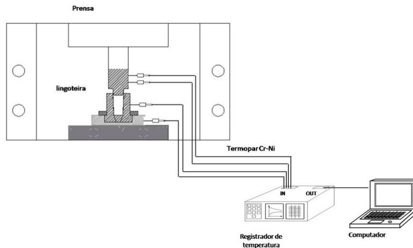
**Figure 2** - Position of thermocouples to obtain temperature.
