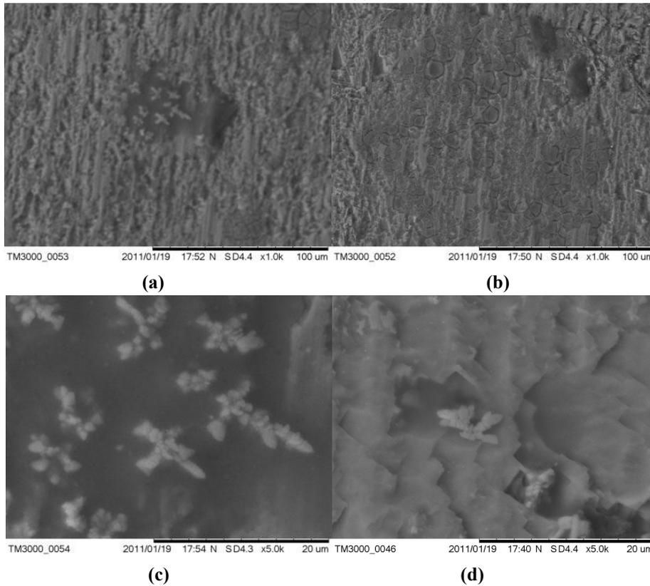
**Figure7** - Microstructure solidified with pressure of 40 MPa (a) 1000X (b) 1000X (c) 5000X (d) 5000X. MEV
