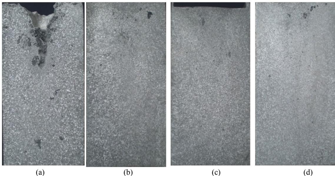
**Figure 4-** Macrostructure Alloy Al-2, 5wt% Mg: (a) Without pressure, (b)40 MPa, (c) 80 MPa and (d) 120 MPa.
