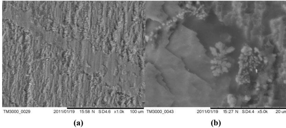
**Figure 9** - Microstructure solidified with pressure of 120 MPa (a) 1000X (b) 5000X. MEV
