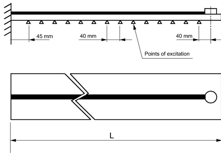
Figure 1. Experimental Modal Analysis setup for the wing model
