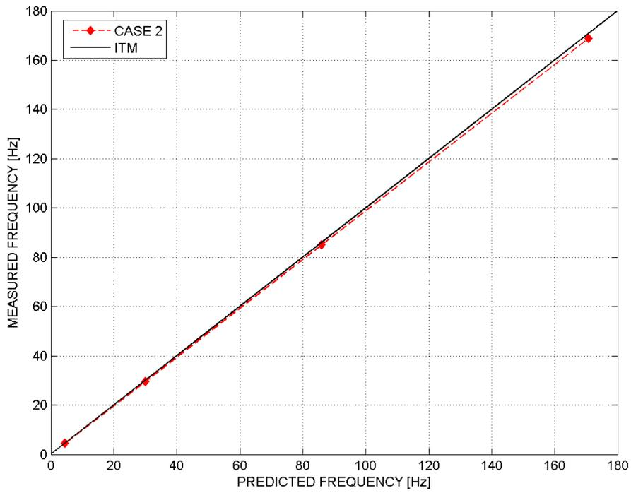
Figure 6. Predicted and Measured comparison - Case 2
