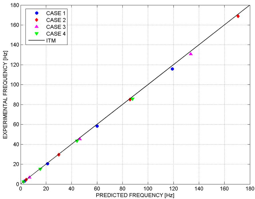
Figure 9. All cases - predicted and Measured comparison
