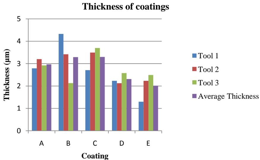
Figure 3. Average values of thickness of the coating of tools.
