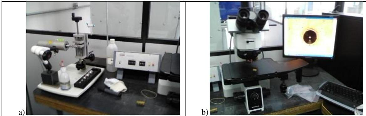
Figure 2. (a) Method of abrasive wear Calotest, (b) Stereoscopic microscope Olympus MX 51.
