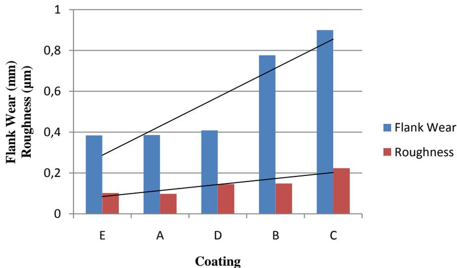
Figure 9. Effect of coating type on the flank wear and surface roughness of the machined material.
