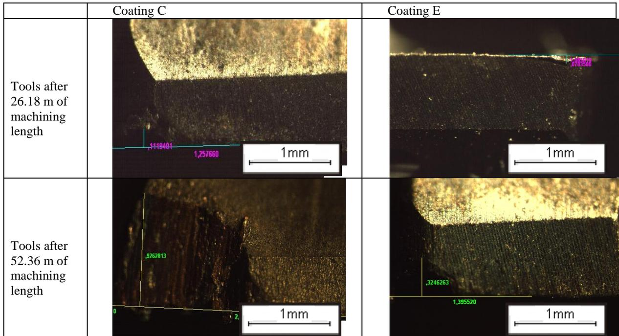
As mentioned in Tab. 3, was also measured the roughness of machined surfaces after machining length of 52.36 meters. The parameter of the surface quality of the work was adopted for the Ra, which corresponds to the average value between the peaks and valleys of the surface in a long analysis, which for the experimental procedure was equivalent to 0.8 mm. Of the amounts collected in surface roughness was obtained for the average roughness of each coating tool used in the experiment, as Fig. 7.
