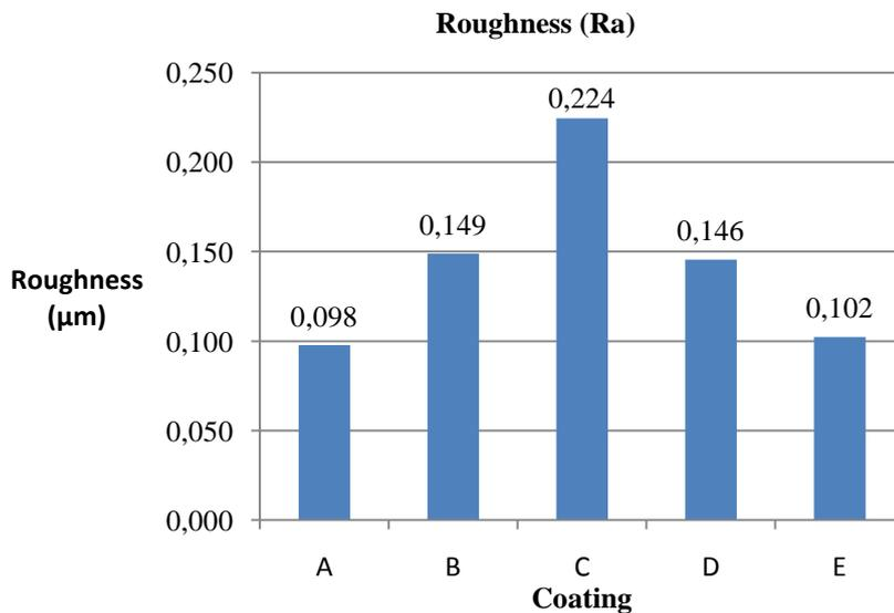
Figure 7. Ra roughness values for the machined surfaces.
