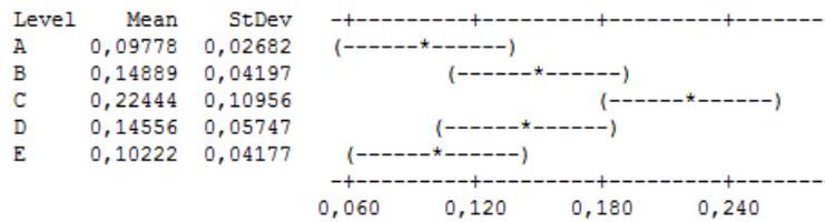
Figure 8. Standard deviation of surface roughness with each coating tool.
