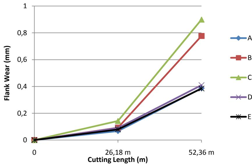
Figure 4. Evolution of flank wear with cutting length.
