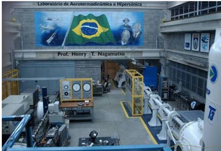
Figure 8. Prof. Henry T. Nagamatsu Laboratory of Aerothermodynamics and Hypersonics. Hypersonic Shock Tunnel T1 (next to the right wall), Hypersonic Shock Tunnel T2 (visible at the left of the Hypersonic Shock Tunnel T3).
