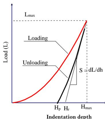
Figure 5 – Aspect of instrumented indentation test
