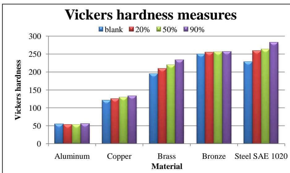
Figure 8. Vickers hardness measures as function of material an homogeneous strain accumulated
