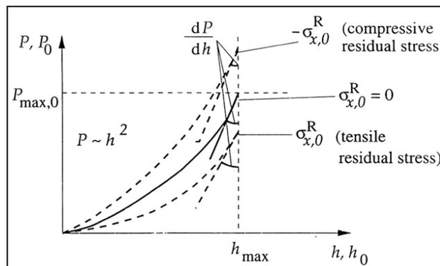
Figure 2. Hardness behavior on presence of residual stress
