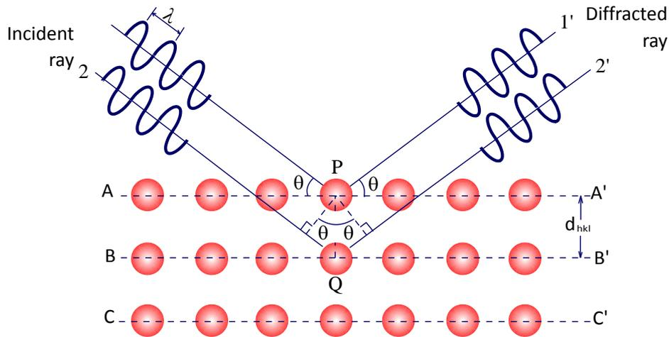
Figure 1. Illustration of the Bragg's theory.
