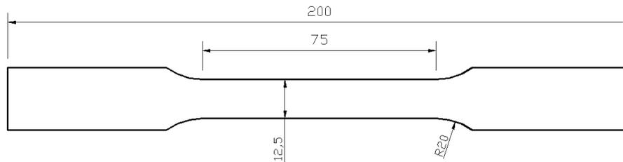
Figure 3. Dimensions of the samples. according to NBR 6152.
