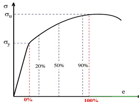
Figure 4. Homogeneous plastic strain - points of study
