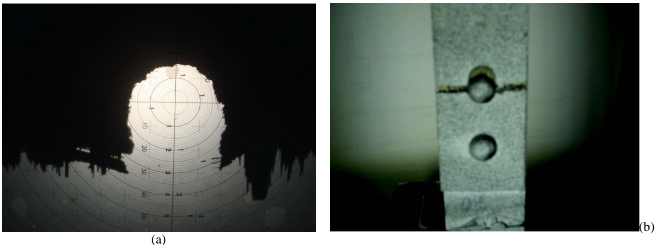
Figure 4. Composite 1: (a) Inelastic strain of the hole -"bearing"; (b) Separation of composite material due to effect of bearing-bypass (net-tension)
