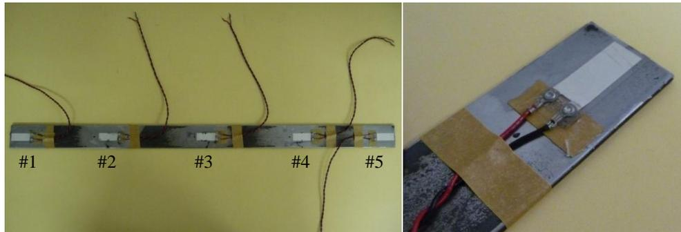
Figure 3.1 – Beam with the five PVDF(s) sensors bonded.
