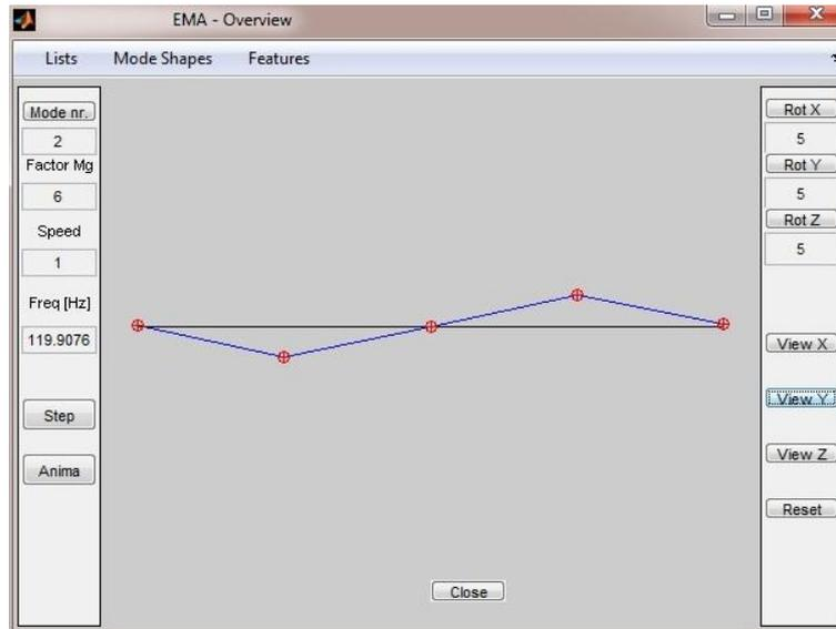
Figure 4.2 – Second vibration mode using a PVDF sensor and Impact Hammer actuator.
