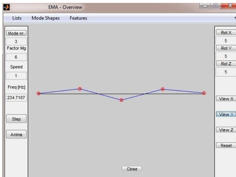
Figure 4.3 – Third vibration mode using a PVDF sensor and Impact Hammer actuator.
