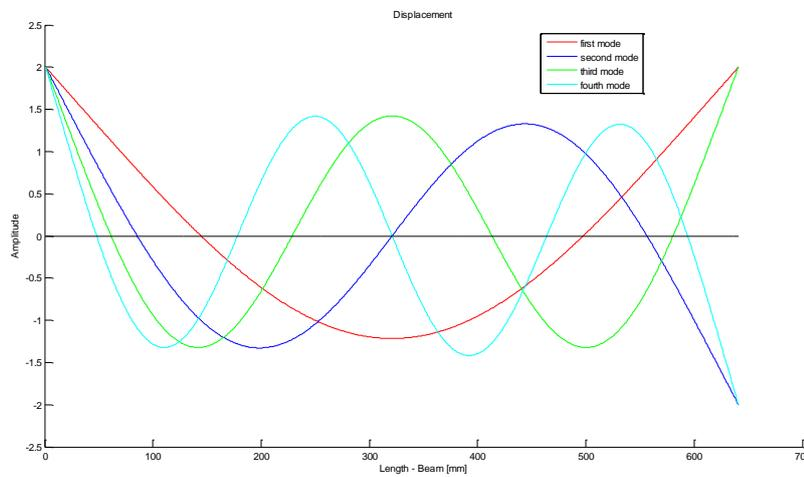
Figure 2.1 – Vibration modes for a continuous free-free beam (displacement).
