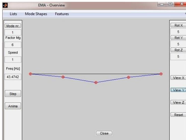
Figure 4.1 – First vibration mode using a PVDF sensor and Impact Hammer actuator.
