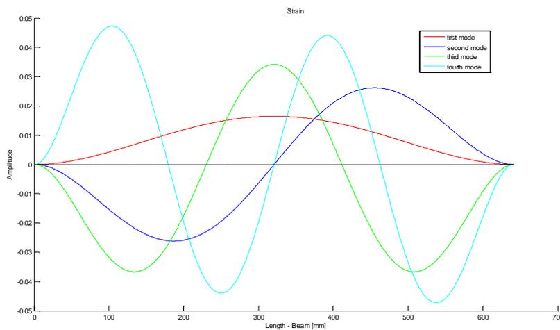
Figure 2.2 – Vibration modes for a continuous free-free beam (slope difference).
