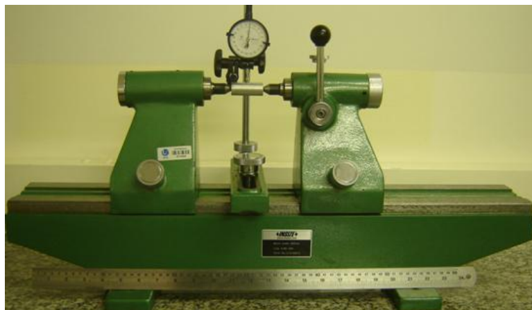
Figure 2. Dial gauge attached to a tailstock device.
