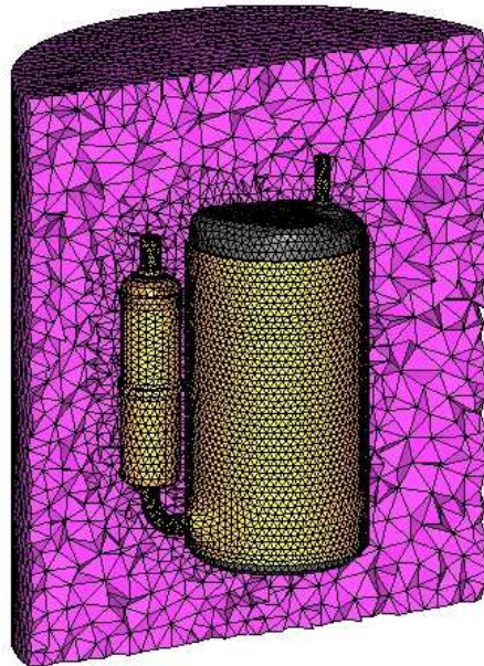
Figure 2 - Acoustic finite element model of the rotary compressor.
