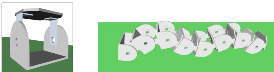
Figure 12. Simulation model of the module and the Pitch-Pitch serpentine system.
