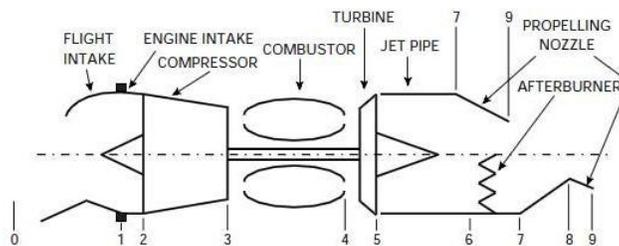
Figure 2. Conventional turbojet, and afterburning turbojet with con-di nozzle (Walsh and Fletcher, 2004).
