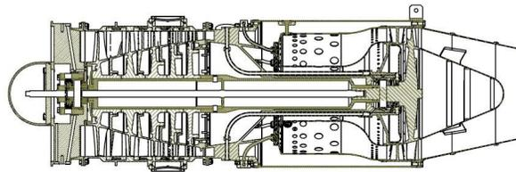
Figure 5. Turbojet engine cross-section (Courtesy TGM Turbines).
