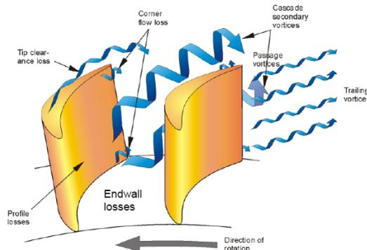
Figure 1. Schematic drawing showing tip clearance loss region (Japikse, 2009)
