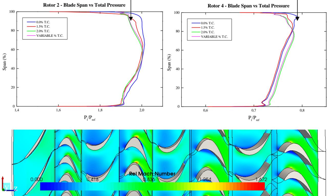
Figure 8. Mach number contours at 90% of blade span.
