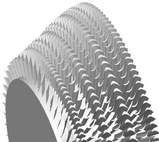
Figure 3. Four-stage axial turbine reconstructed from Leach *et al.* (1982).
