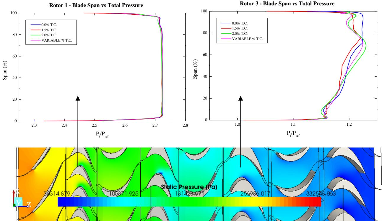
Figure 7. Static pressure contours at 90% of blade span.
