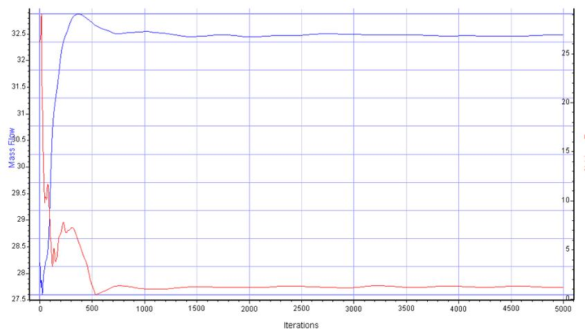
Figure 6. Mass-flow calculations during 5,000 iterations (simulation without tip gap).
