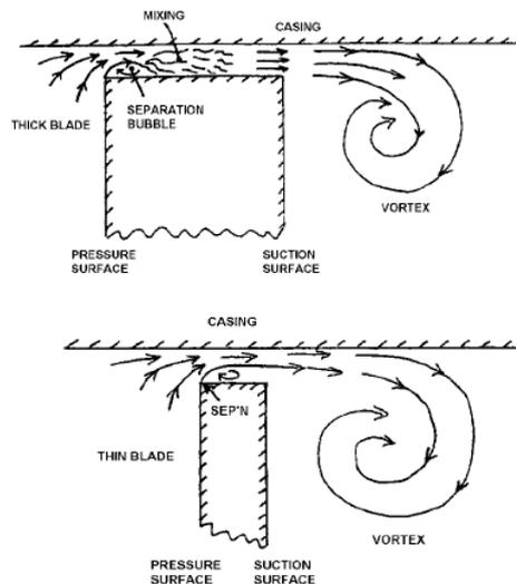
Figure 2. Representation of flows in the tip gap of an unshrouded blade (Denton, 1993)
