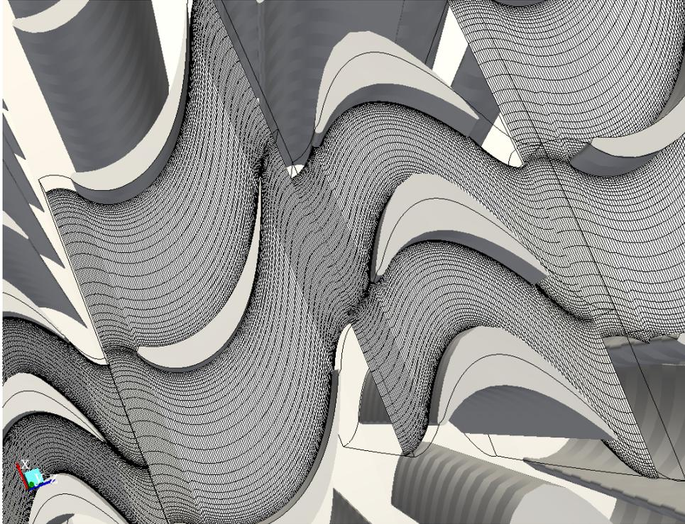
Figure 4 - Generated grid for second stage
