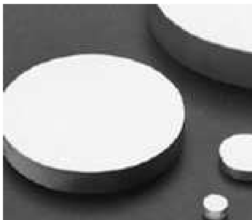
Figure 1. Measurement Standards made from Zerodur®.
