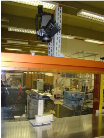
Figure 5a. Detail of the IR camera installation
