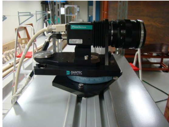
Figure 7. Detail of the PIV laser camera
