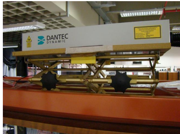
Figure 5b. Detail of the PIV laser positioning
