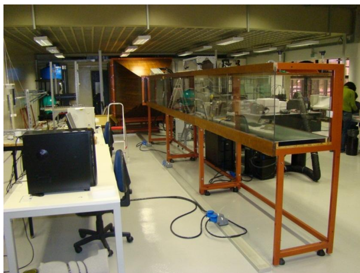
Figure 4. Open circuit blower type wind tunnel of DINAM-INMETRO.
