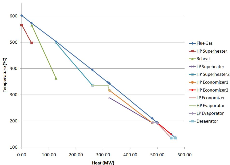
Figure 4 – Cooling curve for the HRSG of the IGCC cycle.
