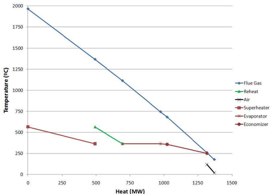
Figure 2 – Cooling curve for the HRSG of the Rankine cycle.
