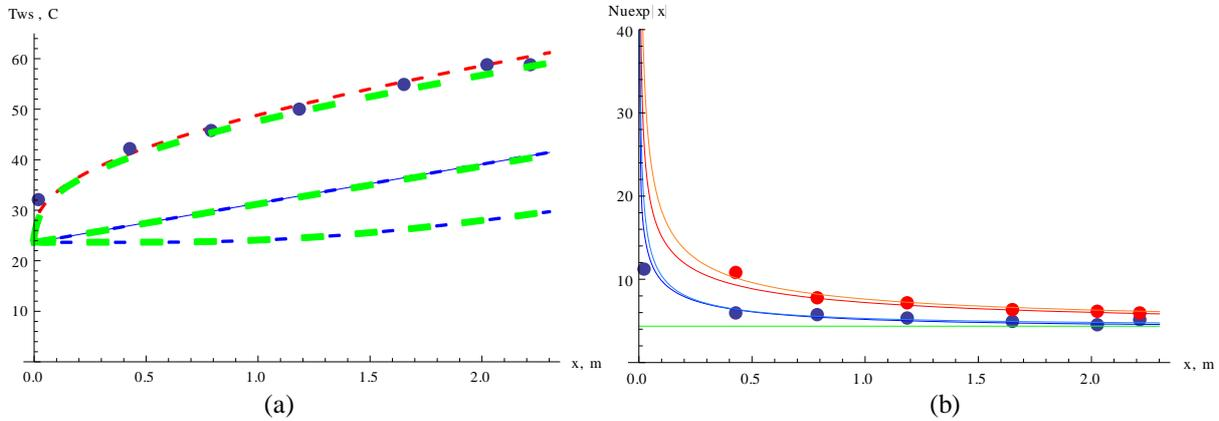
Figures 5.a,b. Experimental and theoretical results (linear and nonlinear models) for (a) wall, bulk and centerline temperatures and (b) local and average Nusselt numbers, for pure water in laminar flow with  $Re = 1531$ .
