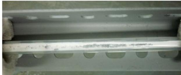
Figure 4. Sedimentation of alumina nanoparticles along the acrylic tube placed after the test section for flow visualization.
