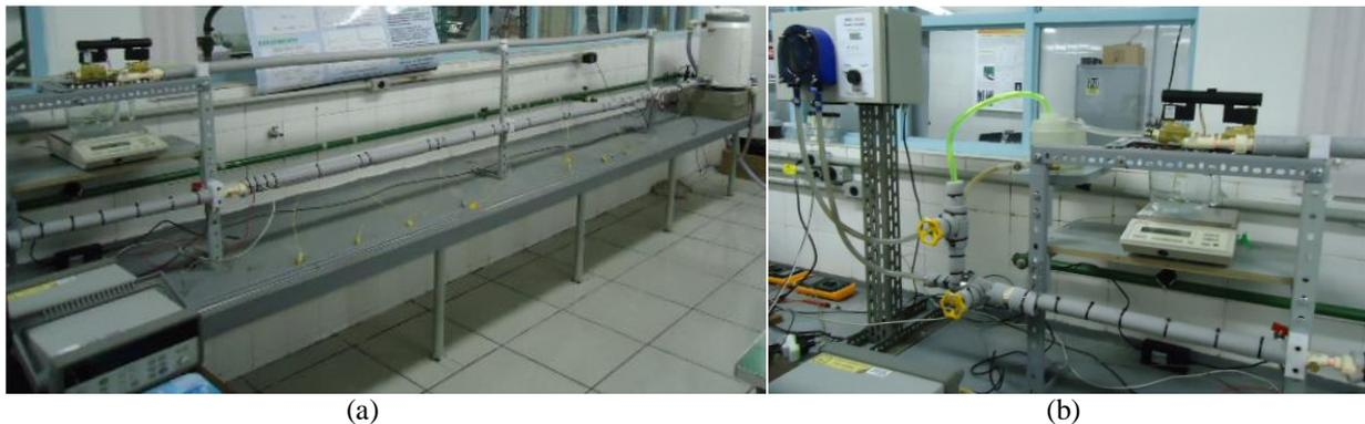
Figures 2. a) Overview of the thermo-hydraulic circuit for experiments on forced convection of nanofluids (LTTTC, COPPE / UFRJ); b) Detailed view of the flow control, pump and mass flow rate acquisition.
