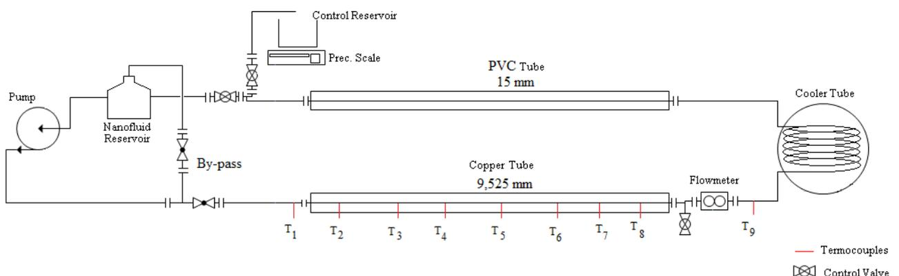
Figure 3. Schematic representation of the experimental apparatus for analysis of forced convection of nanofluids.
