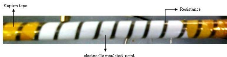
Figure 1. Detail of heater system, with resistance installed over painted copper tube and covered with Kapton tape.
