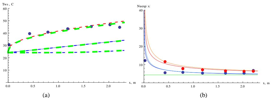
Figures 7.a,b. Experimental and theoretical results (linear and nonlinear models) for (a) wall, bulk and centerline temperatures and (b) local and average Nusselt numbers, for the nanofluid with 2.33% volumetric concentration in laminar flow with  $Re = 1891$ .
