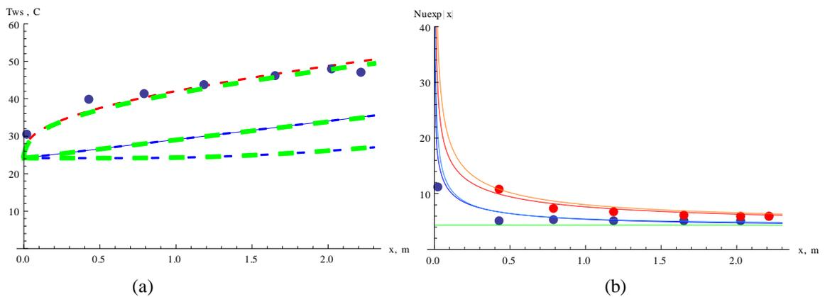
Figures 6.a,b. Experimental and theoretical results (linear and nonlinear models) for (a) wall, bulk and centerline temperatures and (b) local and average Nusselt numbers, for the nanofluid with 3.35% volumetric concentration in laminar flow with  $Re = 1518$ .
