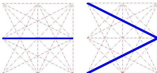
Figure 5. Optimum result of example 2: without (left) and with (right) frequency constraint.
