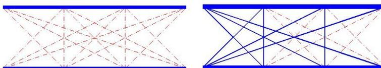
Figure 6. Optimum result of example 3: without (left) and with (right) frequency constraint.
