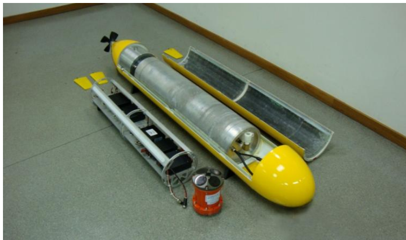
Figure 3. The Pirajuba AUV components. Inside the vehicle, it is shown the manoeuvre and the main vessels. On the left side, the inner platform of the main vessel, and the Doppler Velocity Log (DVL) sensor
