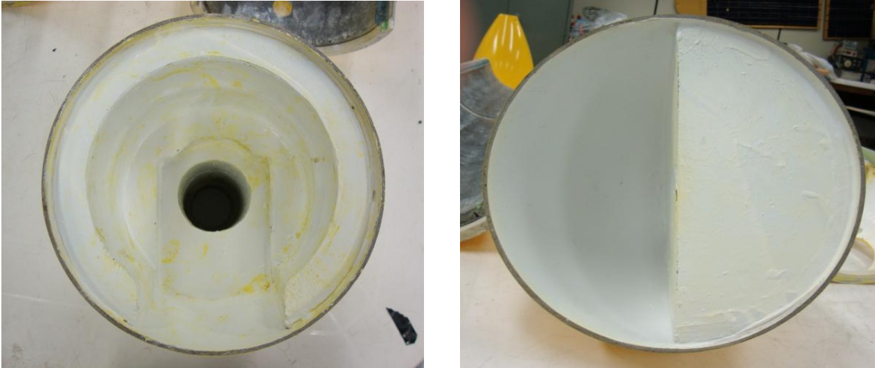
Figure 9. Stern (left side), and bow (right side) filled with the buoyancy foams.
