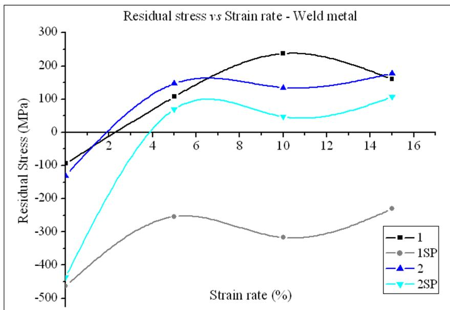
Figure 4. Residual stress average vs strain rate – weld metal.
