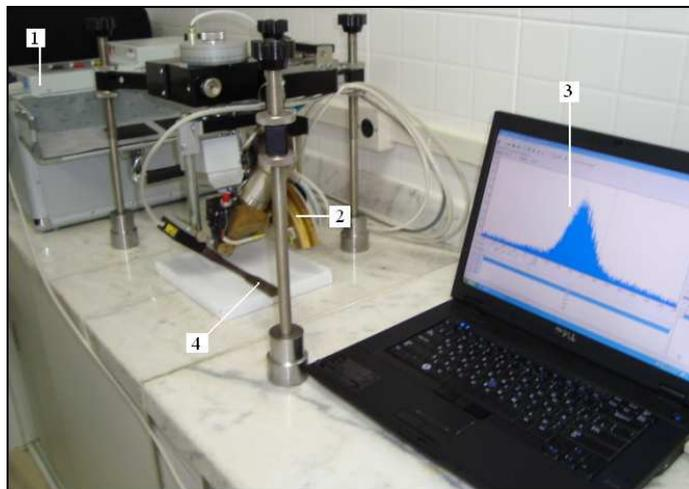
Figure 1. X-rays stress analyzer “Stressrad”: 1 – control unit; 2 – Goniometer; 3 – data acquisition system; 4 – analyzed specimen.
