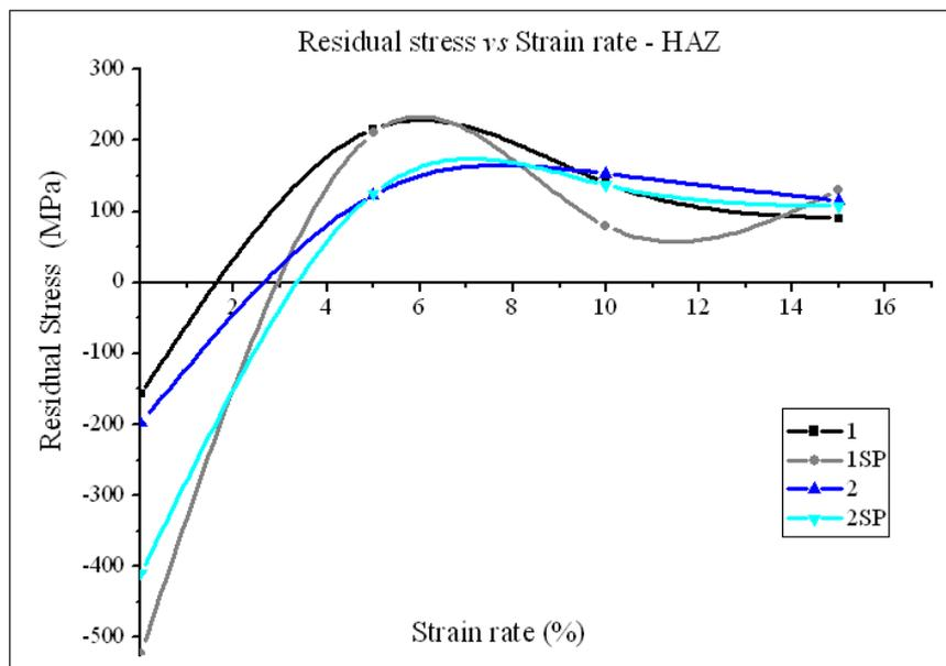
Figure 3. Residual stress average vs strain rate – HAZ.
