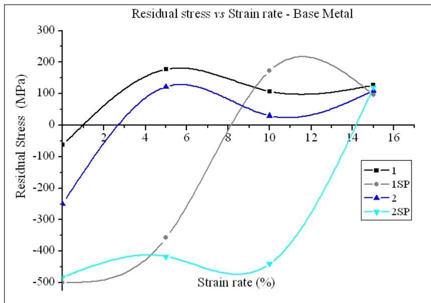
Figure 2. Residual stress average vs strain rate – base metal.
