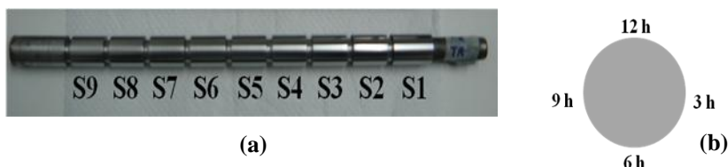
Figure 3. (a) Geometry and (b) longitudinal directions (12h, 3h, 6h and 9h) of roughness and waviness measurement on the AISI 1045 steel rod.
