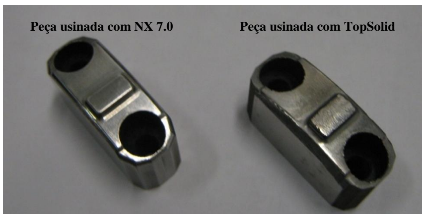
Figura 4 – Puncture machining used on printing engine. At left, the puncture machined with NX 7.0; at right, with TopSolid.
