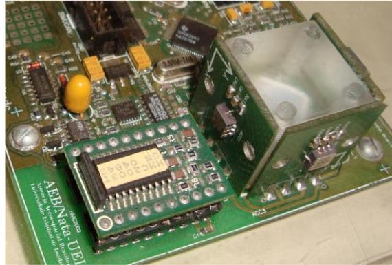
Figure 4. Hardware with triads of MEMS sensors used in calibrations tests
