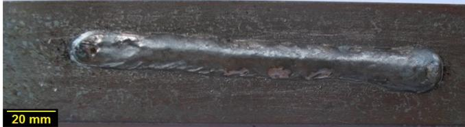
A weld bead with a circular end on the right side. The surface is relatively smooth. A 20 mm scale bar is visible in the bottom left corner.       | 5                                   | 8                       | 8                        | 12            |
