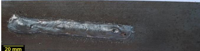
A weld bead with a circular end on the left side. The surface is very rough and irregular. A 20 mm scale bar is visible in the bottom left corner.   | 10                                  | 2                       | 2                        | 5             |
