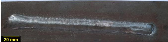
A weld bead with a circular end on the right side. The surface is relatively smooth. A 20 mm scale bar is visible in the bottom left corner.       | 10                                  | 8                       | 8                        | 15            |
