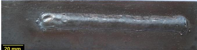
A weld bead with a circular end on the right side. The surface is very smooth and uniform. A 20 mm scale bar is visible in the bottom left corner. | 10                                  | 8                       | 2                        | 20            |
