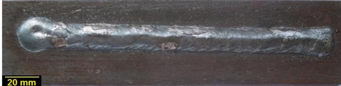
A weld bead with a circular end on the left side. The surface is relatively smooth. A 20 mm scale bar is visible in the bottom left corner.        | 5                                   | 8                       | 2                        | 13            |
