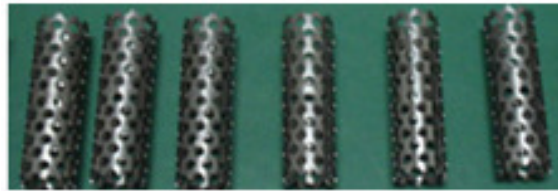
Figure 4. Mesh cages used in fatigue testing.
