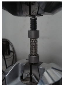
Figure 5 – Mesh cage fixed to MTS clamping jaws.
