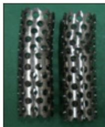
Figure 9. End configuration of two specimens after compression testing.
