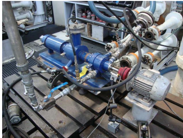
Figure 6. The PAT operating in the pump mode at test facilities of a pump manufacturer.
