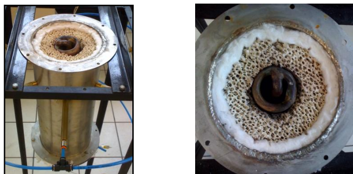
Figure 3. Photo of the burner open surface and the coil positioned in the center of the porous medium.
