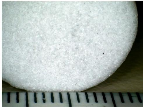
Figure 9. Silica glass-ceramic composed of Amorphous SiO<sub>2</sub> matrix reinforced with alpha-quartz particles.
