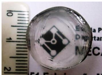
Figure 7. Compact obtained starting from amorphous SiO<sub>2</sub> powder.
