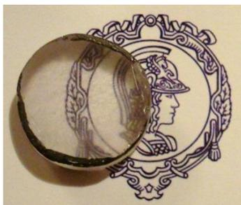
Figure 5. Sample obtained from the sintering of crystalline powder with 60°C/min. of heating rate.
