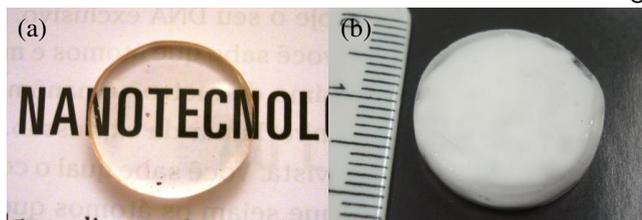
Figure 6. Transparent fused silica obtained from amorphous nanopowder (a). Milky glass due to numerous micro-bubbles (b).
