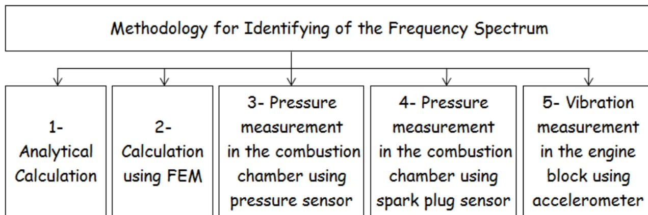
Figure 2. Methodology for characterization of the single cylinder research engine
