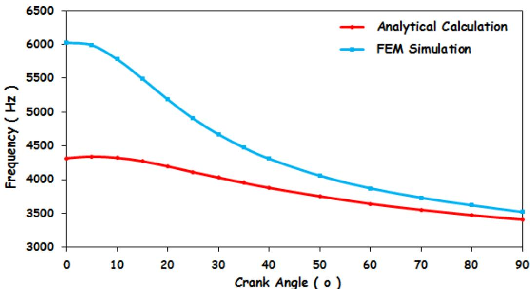
Figure 3. Comparison of analytical calculation and FEM simulation results
