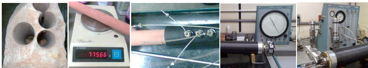
Figure 3. Botucatu Sandstone, weight, coreholder insert, Porosimeter and Permeabilimeter.
