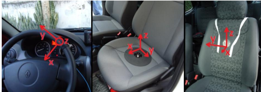
Figure 5. Coordinate system for seat pad and accelerometer measurements.
