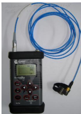
Figure 4. VI400-Pro equipment and accelerometer used in measurements.
