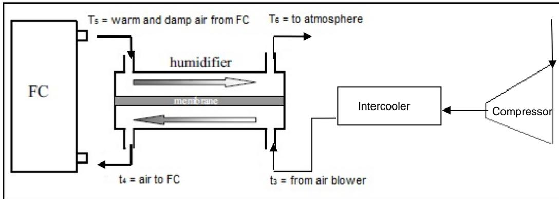
Figure 1. Humidification system using the exit air.
