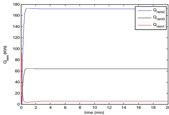
Figure 8. Removed heat.
