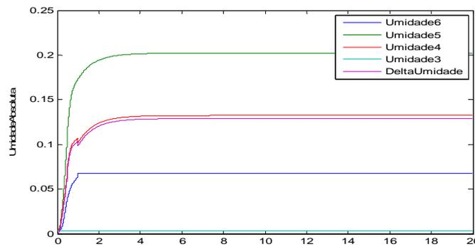
Figure 4. Variables without extra humidification in PEMFC.
