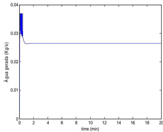
Figure 13. Water flux in PEMFC *versus* time.
