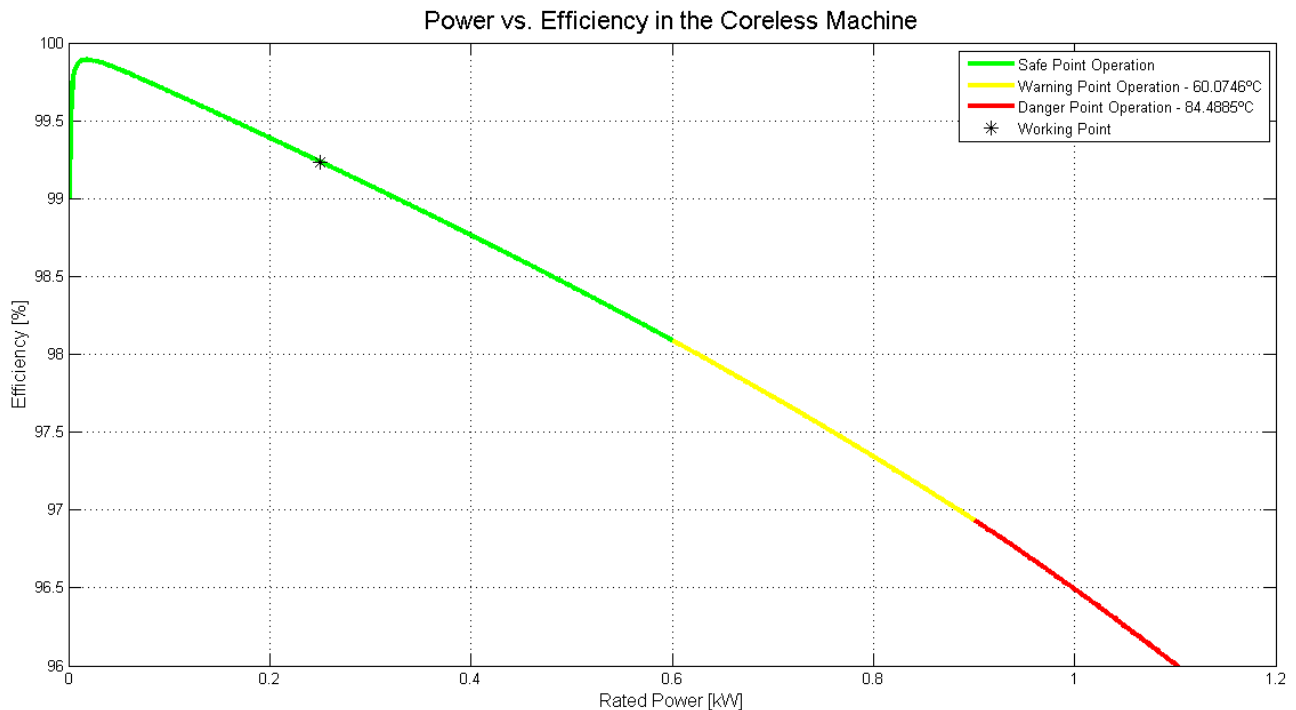
Figure 5 – Power capability restricted by the temperature rise
