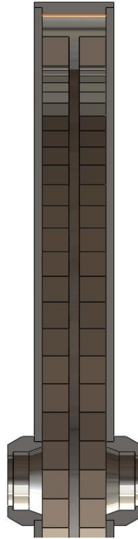
Figure 8 – Section view of the rotor
